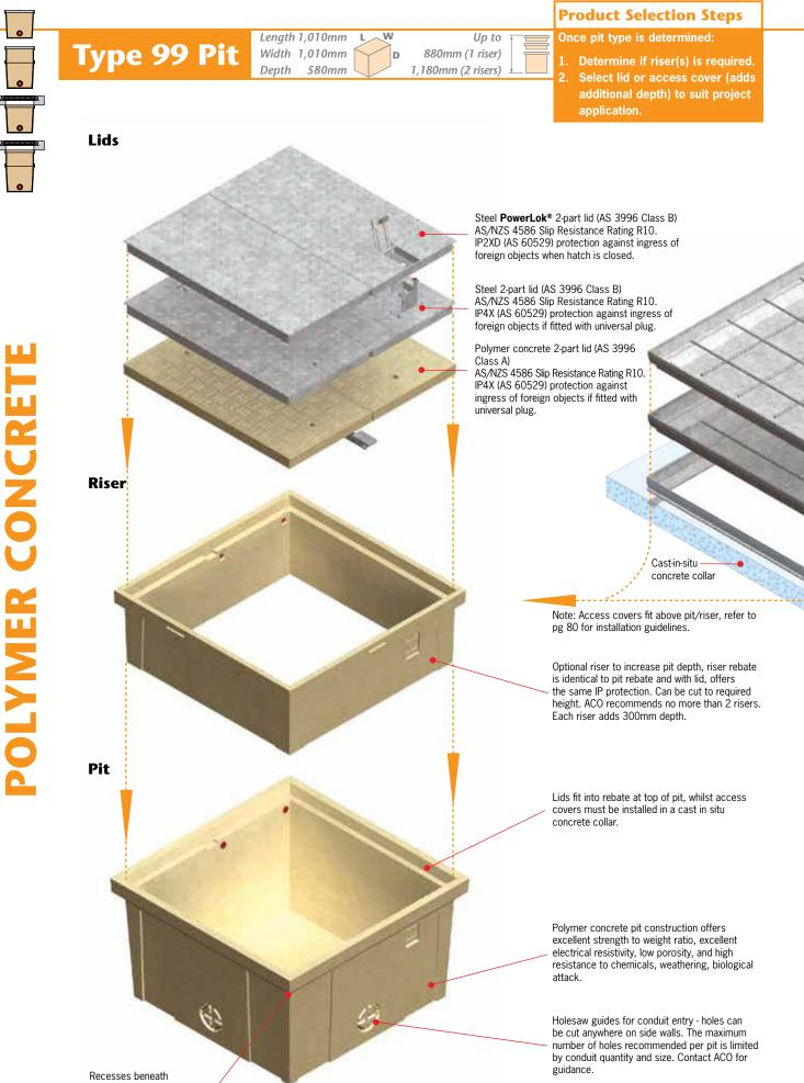
Recesses beneath rebate on opposite corners to fit ACO's lifting device. See page 43.
